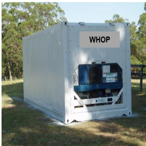
Waste Heat to Osmotic Power Module
